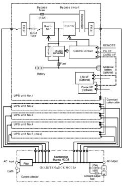
Fig. 7 System Circuit Block Diagram
